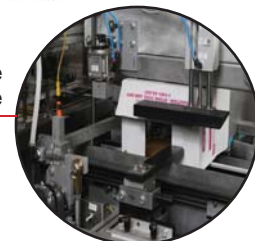
Horizontal Case Erecting and Discharge
