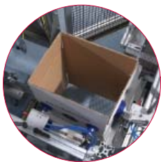
Reliable case opening with opposing vacuum system
