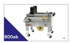
3M-Matic™ Case Sealer 800ab is an adjustable side belt drive case sealer. Applies bottom seal only at rates up to 40 cases per minute, using tape widths from 36mm to 48mm, and also 72mm tape.
