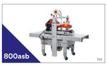
3M-Matic™ Case Sealer 800asb is an adjustable side belt drive case sealer. Seals up to 28 cases per minute, using tape width of 36mm.
