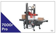
**3M-Matic™ Random Case Sealer 7000r Pro** is a semi-automatic random case sealer that automatically adjusts for case height and width and is capable of sealing 24 cases per minute, using tape widths from 36mm to 48mm wide.
