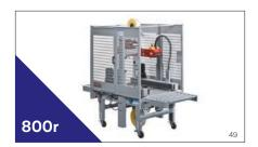
**3M-Matic™ Case Sealer 800r** is a semi-automatic random case sealer automatically adjusts for case height and width. Top and bottom seal at rates up to 20 cases per minute, using tape widths from 36mm to 48mm wide.
